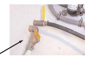
Port & Starboard Overboard Waste Valves
