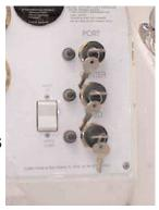
Turn key(s) to the full right start position until the engine starts, and then release the key. It will spring back to the on-run position. **Note:** Do not turn key to the start position with the engine running or starter and/or engine damage may occur.
