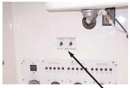
Overboard Discharge Pump Switch
