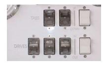
Using the rocker switches on the dashboard above the quadrant, lower the trim tabs to the full down position, as indicated on the trim tab indicators.
