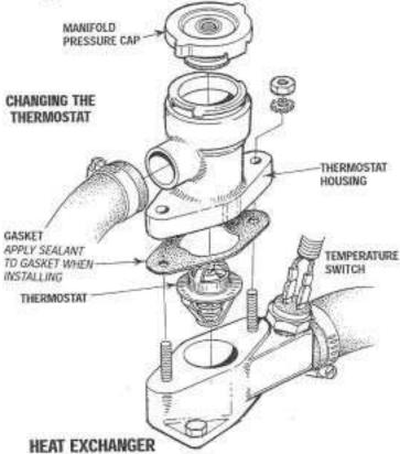
Cool raw water flows through the inner tubes of the heat exchanger. As the engine coolant passes around these tubes the heat of the internal engine is conducted to the raw water which is then pumped into the exhaust system and discharged. The engine coolant (now cooled) flows back though the engine and the circuit repeats itself.
