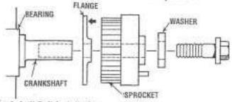
Crankshaft Bolt Installation
