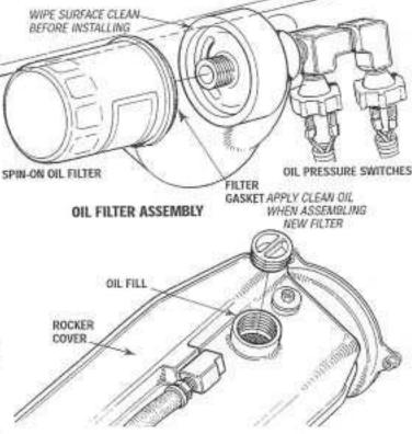
NOTE: Generic filters are not recommended, as the material standards or diameters of important items on generic parts might be entirely different from genuine parts. Immediately after an oil filter change and oil fill, run the engine to make sure the oil pressure is normal and that there are no oil leaks around the new oil filter.
