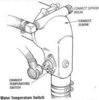
A high water temperature switch is located at the thermostat housing. Normally closed, this switch, should the fresh water coolant's operating temperature reach approximately 210°F (99°C), will open and interrupt the DC voltage to the K2 run relay therebyshutting off the engine. This switch resets at
