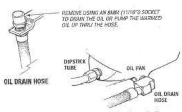
Replacing the Oil Filter. When removing the used oil
