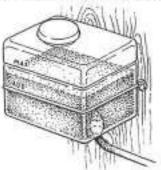
NOTE: Periodically check the condition of the manifold pressure cap. Ensure that the upper and lower rubber seals are in good condition and check that the vacuum valve opens and closes tightly. Carry a spare cap.
