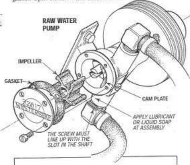
CAUTION: If any of the vanes have broken off the impeller, they must be located to prevent blockage in the cooling circuit. They often can be found in the heat exchanger.
