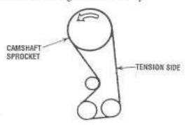
Loosen the temperorarily tightened tensioner nut on the water pump side 1 or 2 turns, and tension the belt making use of spring force.
